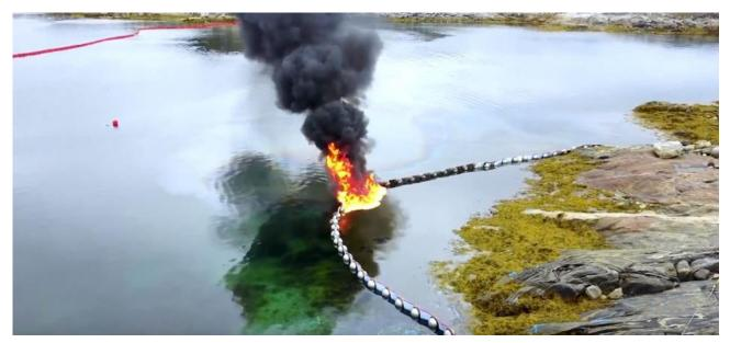
Figure 3. Image of the on-shore *in situ* burning of naphtenic North Atlantic crude oil after the fire was ignited. (footage from the video "Combat of oil spills in Arctic waters - in situ burning experiments, Greenland. Summer 2017. GRACE" <u>https://youtu.be/51ieM7h7ykM</u>)
